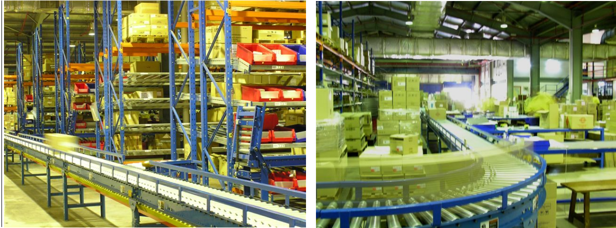
Pharmaceutical Warehouse Picking and Packing Layout
